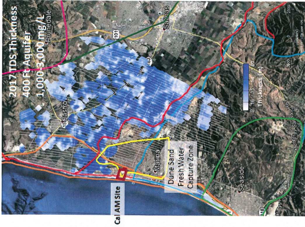
Figure 4-104. Comparison of the TDS distribution and thickness for the TDS range of 1,000-3,000 mg/L in the 400-Foot Aquifer from the 2017 (left image) and 2019 (right image) AEM surveys within the bounds of the 2017 AEM survey.
