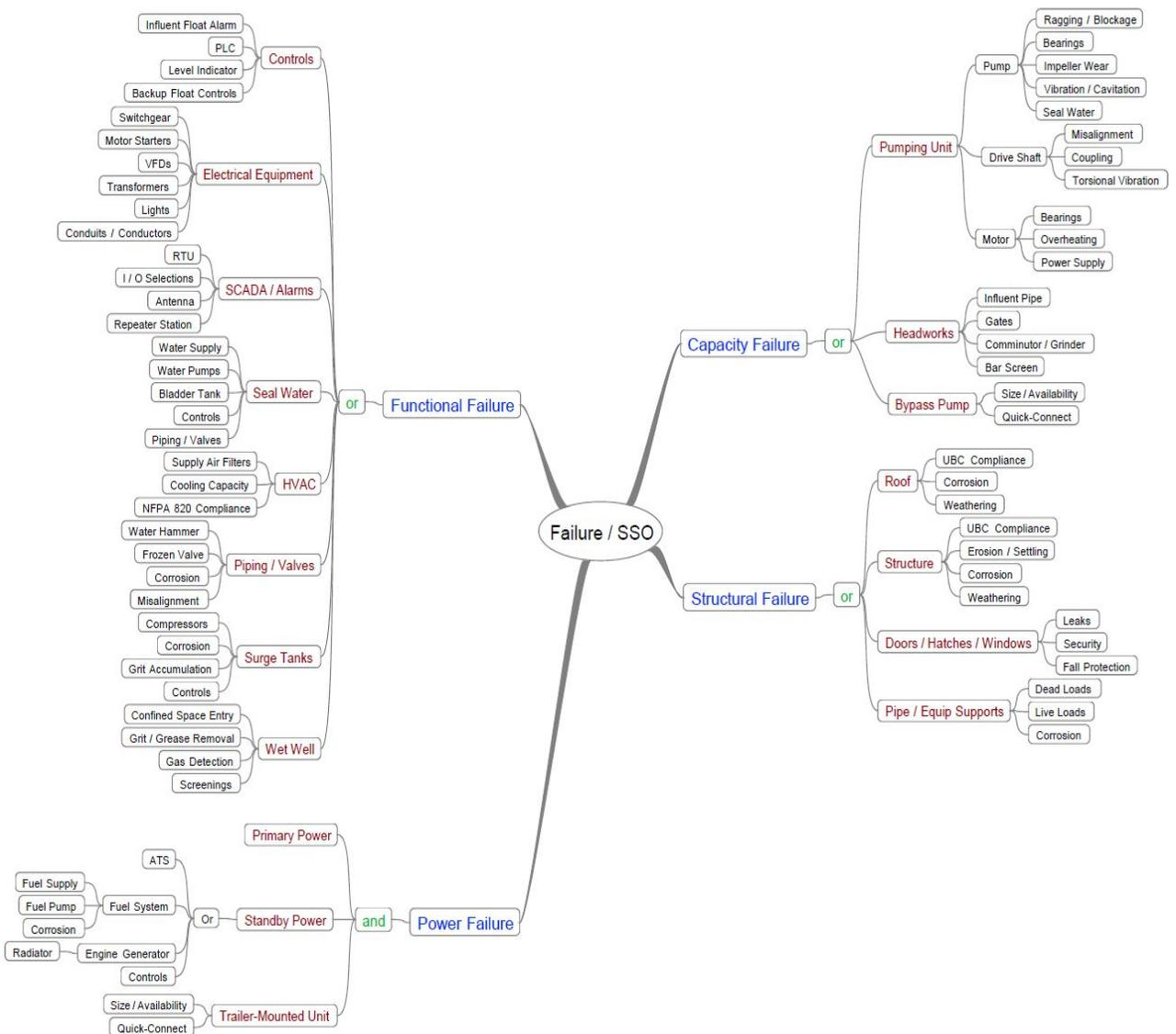
Categories of failure include Functional, Power, Capacity, and Structural. The diagram flowchart shows how specific variables of the lift station (black text) contributes to a general variable (red text), which can lead to a type of failure (blue text) that ultimately can lead to a sanitary sewer overflow (SSO). As an example from the
